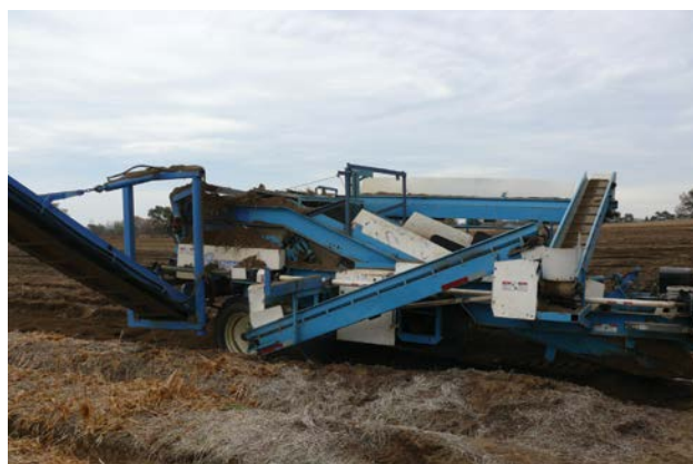
Figure 102. Fully automated ginseng harvester.
