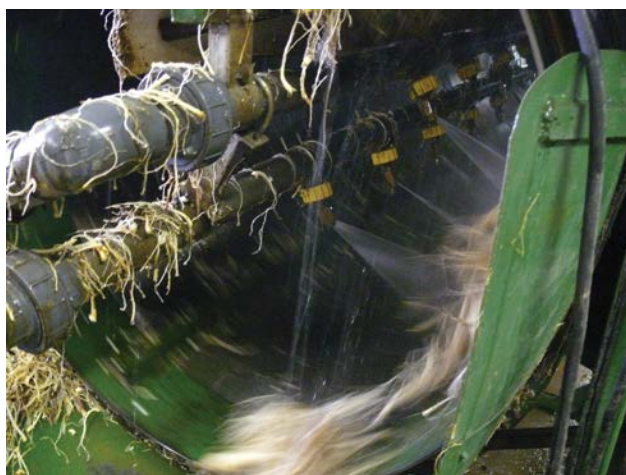
Figure 107. Root washing drum, often used as part of the washing line.
