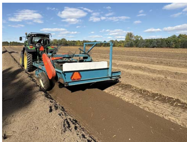
Figure 103. A modified potato digger placing roots onto the surface of the soil for either hand harvest or further machine harvest. This machine is usually followed by a crew of workers to manually collect any roots missed by the machine
