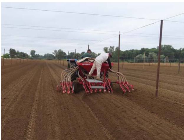
Figure 27. An air-assist seeder used to seed ginseng.
