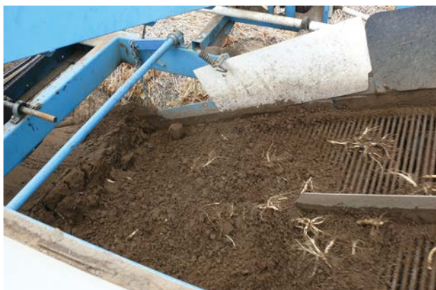
Figure 101. A modified potato digger undercutting a ginseng bed. The soil and root mixture rides up a conveyor of metal slats causing the soil to fall through and any root or larger debris to ride up the conveyor, ending up on top of the soil.
