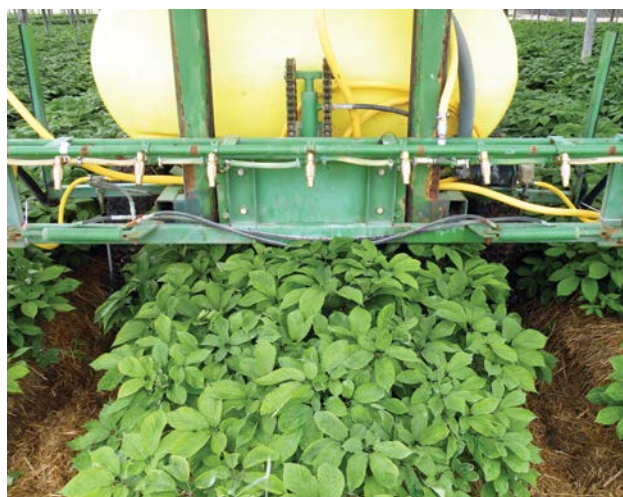
Figure 99. Custom-made ginseng sprayer. A standard design in Ontario.
