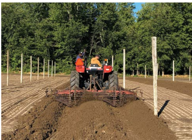
Figure 23. A bed groomer used to smooth out the beds after bed forming.
