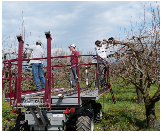
Figure 5. Platform that can be used to increase labour efficiency by reducing the need for ladders.
