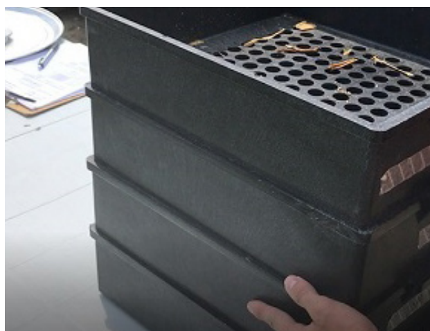
Figure 14-4. Penn State Shaker Box used to measure particle size distribution in ruminant rations
