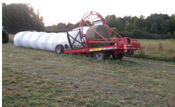
Figure 15-6. An in-line wrapper.
