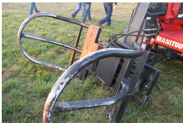
Figure 15-5. A grapple minimizes punctures in the plastic wrap.
