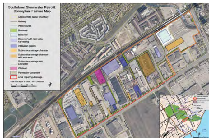
Figure B5-25. Southdown – the engineer's conceptual design of the Southdown stormwater retrofit.
